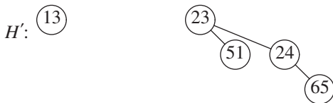
Figure 6.47 Binomial queue H' , containing all the binomial trees in H_3 except B_3
