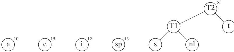
Figure 10.15 Huffman's algorithm after the second merge
